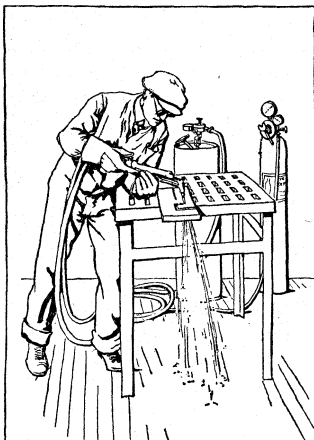
BY COURTESY OF LINDE AIR PRODUCTS CO CUTTING METAL WITH AN OXY-ACETYLENE FLAME, ONE OF INDUSTRY'S MANY USES OF ACETYLENE
